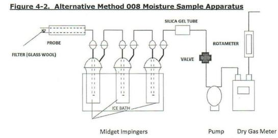
\*The silica gel tube depicted in the figure above was replaced with a midget impinger (bubbler) with a straight tube insert, as allowed in ALT-008, §1.
