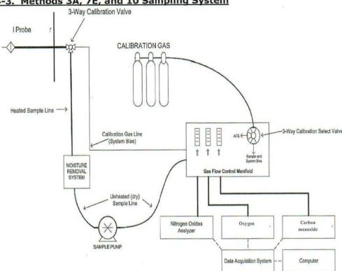
Figure 4-3. Methods 3A, 7E, and 10 Sampling System
