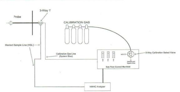
Figure 4-6. USEPA Method 25A NMOC Sample Apparatus
