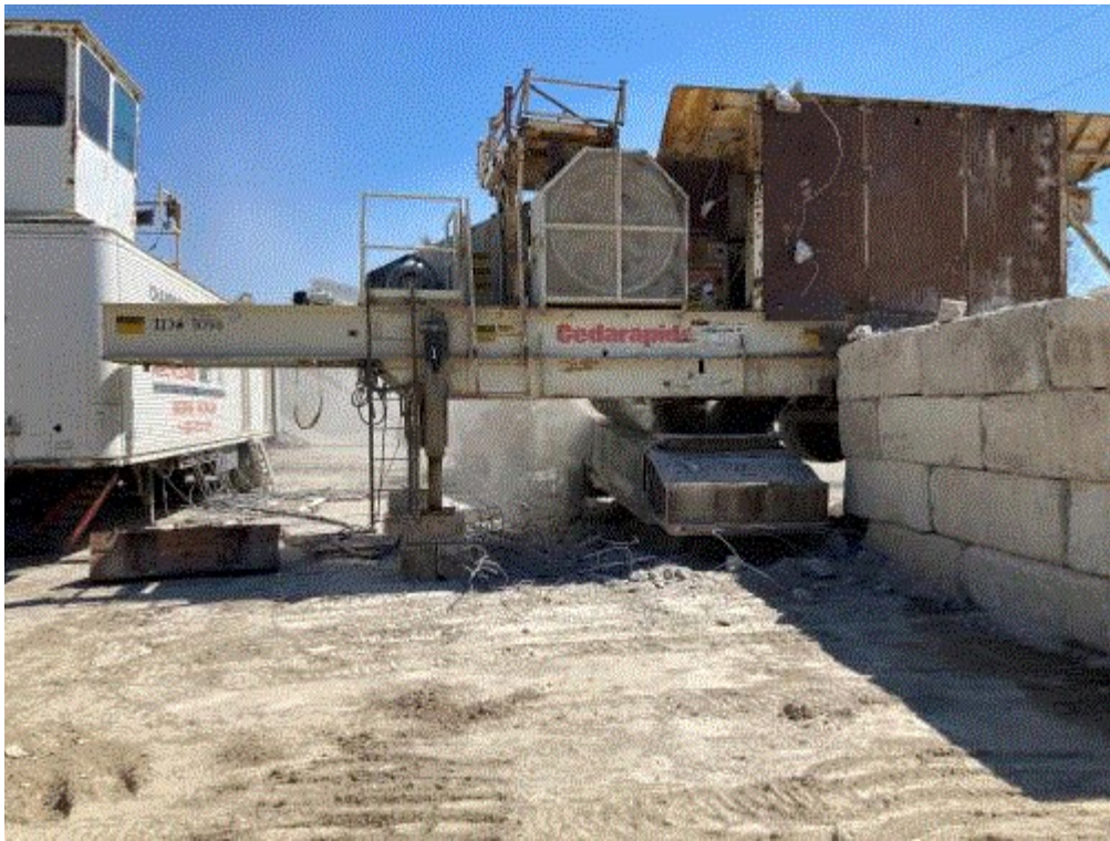
Image 1(001) : Fugitive dust from primary crusher.
