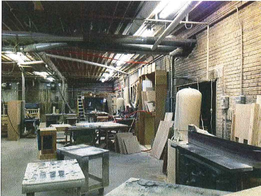
Image 5(CF3) : Wood waste collection system
