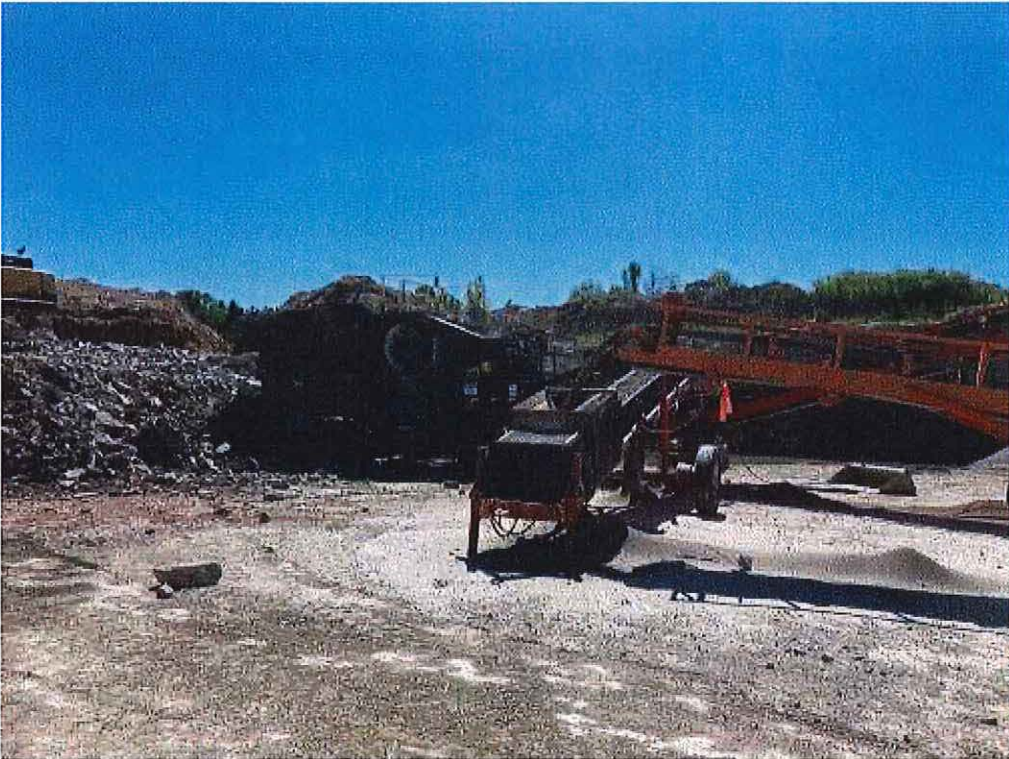
Image 2(Primary) : Primary jaw crusher.
