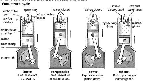
Figure 3-1. Four-Stroke Engine Process Diagram
