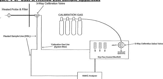
Figure 4-6. USEPA Method 25A Sample Apparatus
