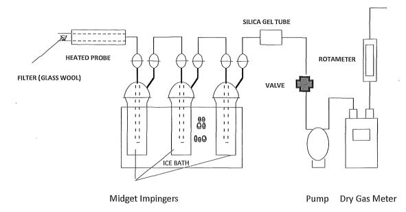
The silica gel tube depicted in this figure was replaced with a midget impinger (bubbler) with a straight tube insert, as allowed in ALT-008, §1
