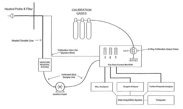
Figure 4-4. USEPA Methods 3A, 7E, and 10 Sampling System
