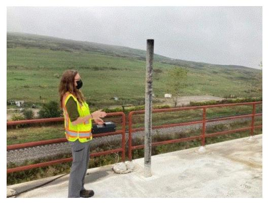
**Image 2(Passive vent) :** Passive vent from condensate sump. Measured methane at 129,000 ppm with measured H2S greater than 50 ppm.
