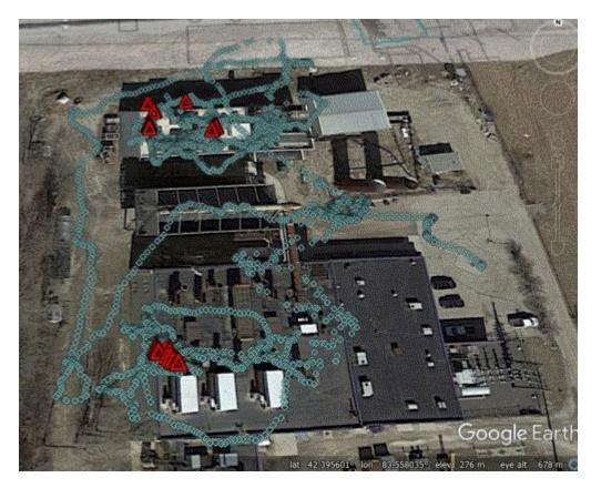
**Image 5(Map 3) :** Red triangles show where methane concentrations exceeded 500 ppm.
