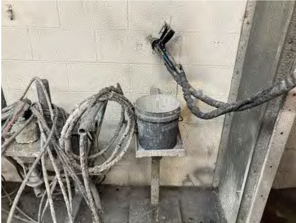
Image 6(FGELCOAT) : Open acetone waste bucket in FGELCOAT booth.
