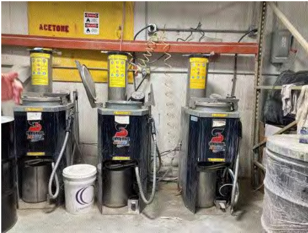
Image 2(Acetone Recycling) : 3 acetone recyclers used for waste acetone.
