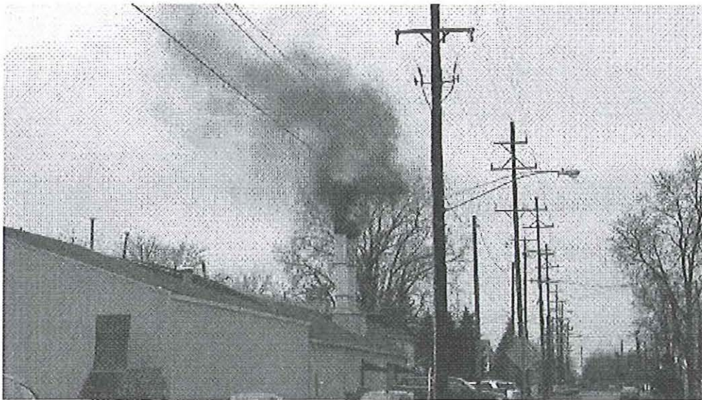
Image 2(Looking West) : Opacity from Unit #2. Observer standing East of the facility. Time taken 10:06. glm
