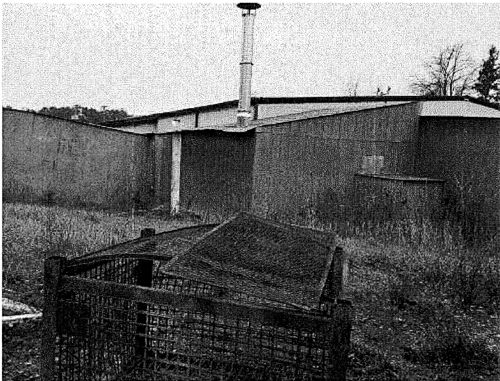
Image 8(Metal cage) : Metal cage used to burn wooden pallets. In the background is the stack for the burn-off
