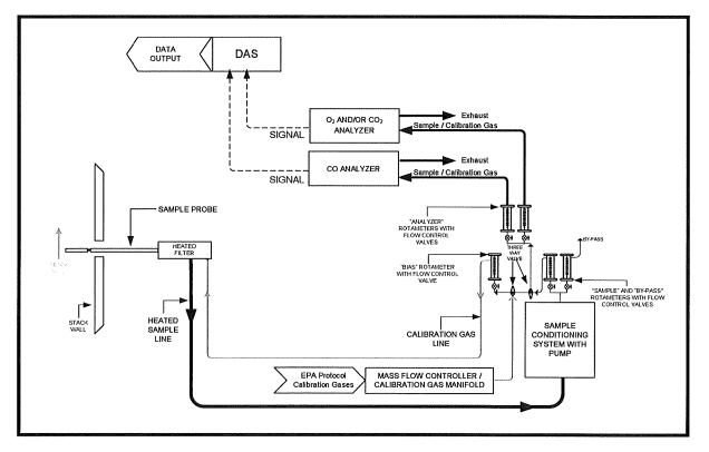
FIGURE 3-1 EPA METHODS 3A AND 10 SAMPLING TRAIN
