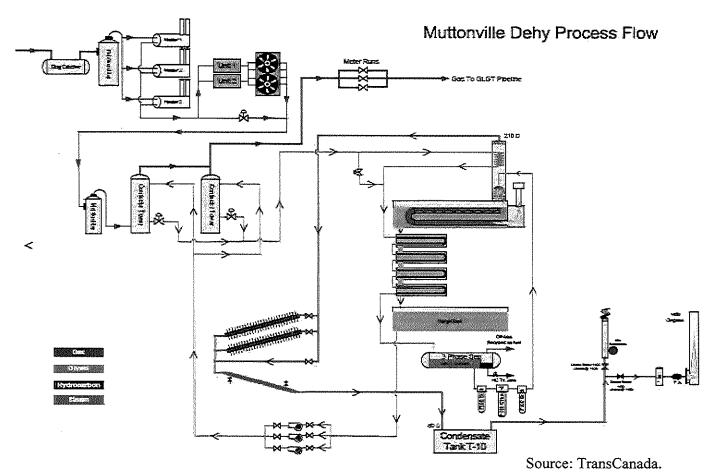
Figure 2-2. Muttonville Dehydration Unit Process Flow
