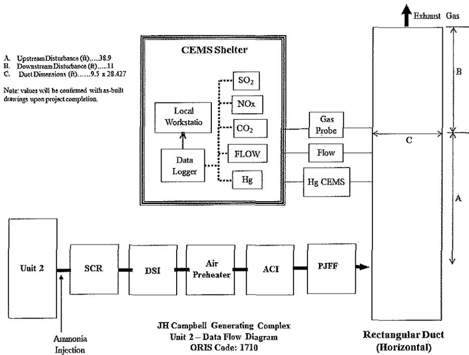
Figure 3-1: Unit 2 Process Schematic (July - DSI before Air Heater)
