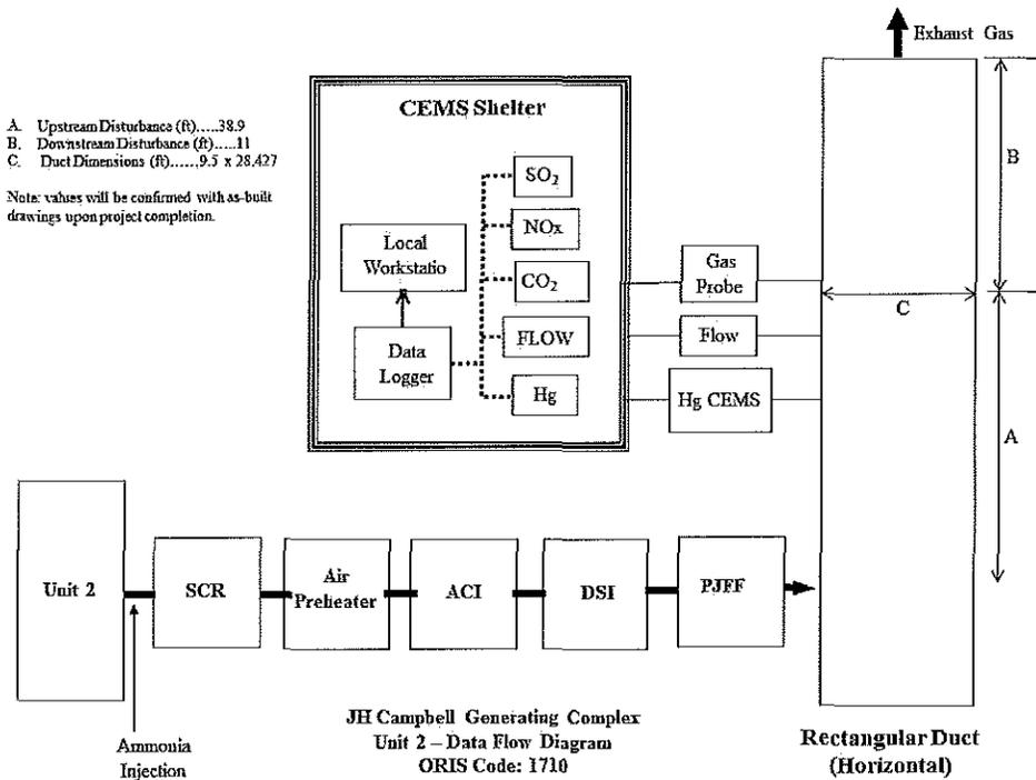
Figure 3-2: Unit 2 Process Schematic (August - DSI after Air Heater)
