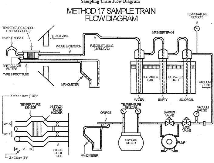
Figure 2 Sampling Train Flow Diagram
