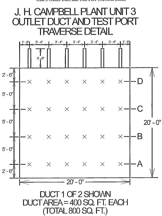
Figure 4 Unit 3 Outlet Duct and Test Port Traverse Detail
