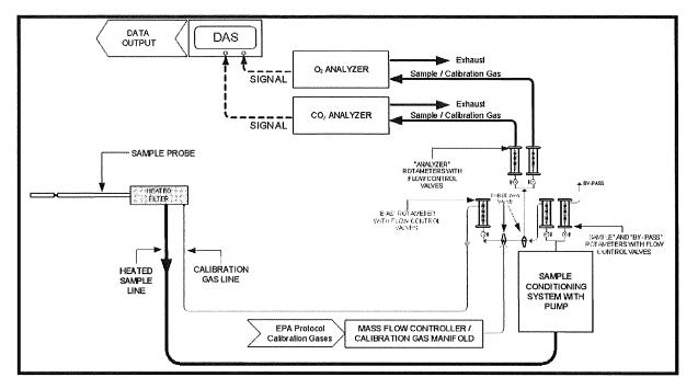
FIGURE 3-1 EPA METHOD 3A SAMPLING TRAIN
