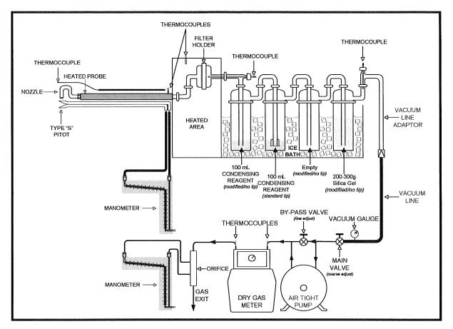
FIGURE 3-2 EPA METHOD 5 SAMPLING TRAIN
