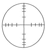
Figure 3 – Sampling Location St.Clair Power Plant - Unit 7 266' Stack Diameter 192" Sampling Ports >2 Duct Dia. >8 Duct Dia. 2821 Flow ESP
