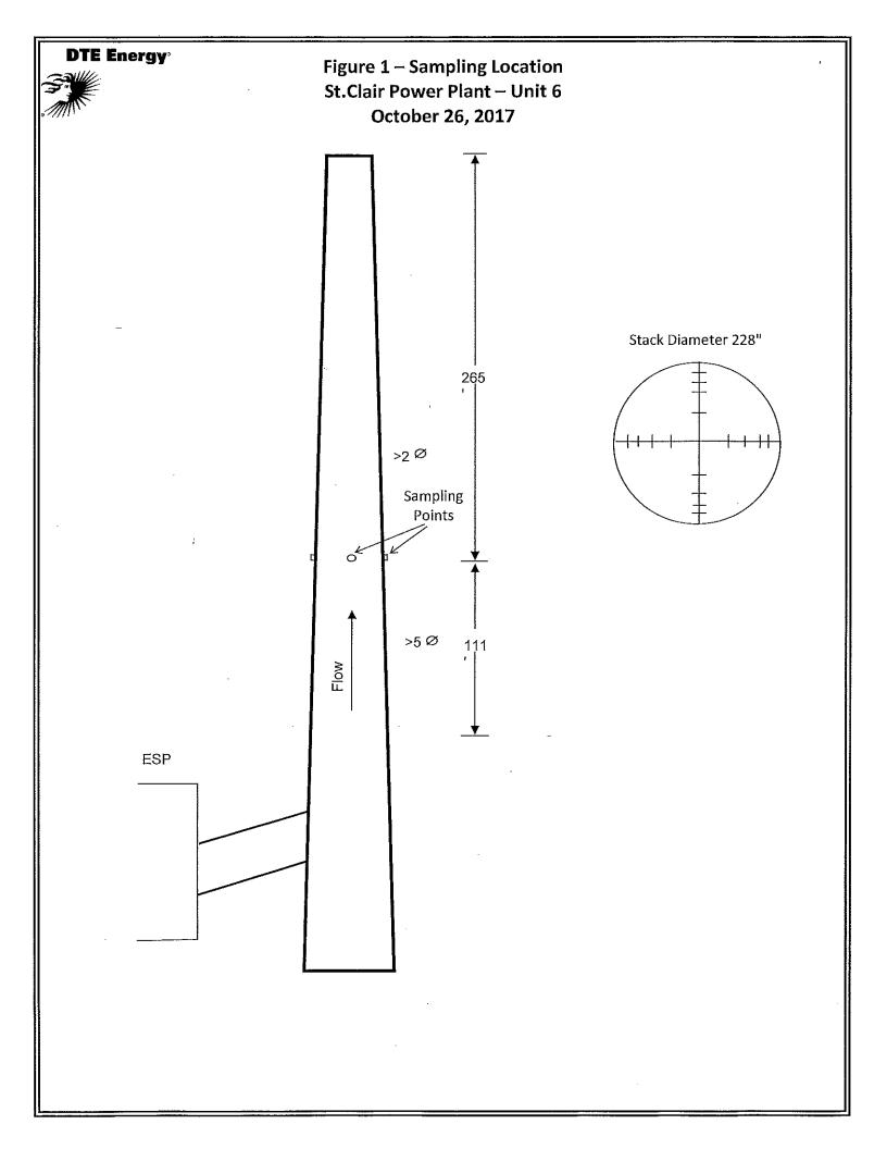
Figure 2 – ASTM D6348 St.Clair Power Plant – Unit 6 October 26, 2017
