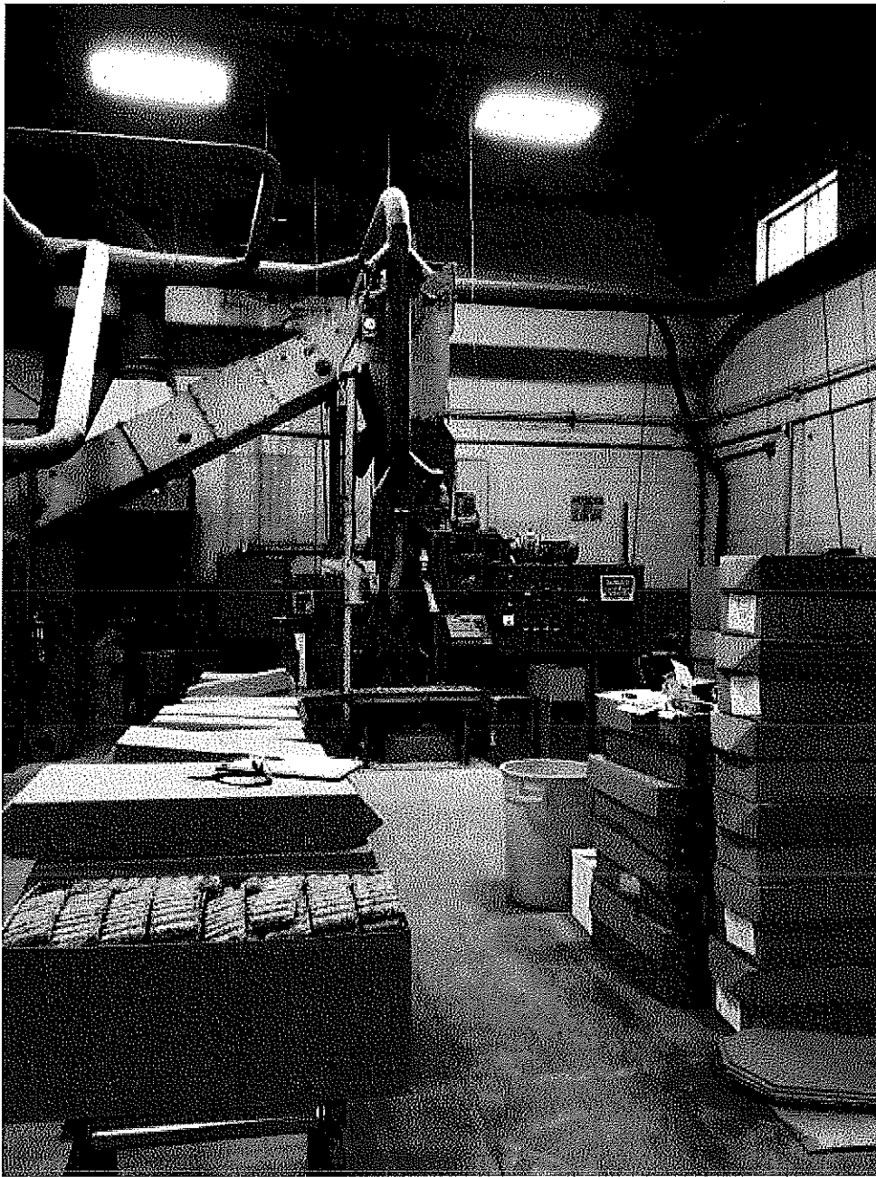
Image 7(15) : Compound mixing process - briquetter.
