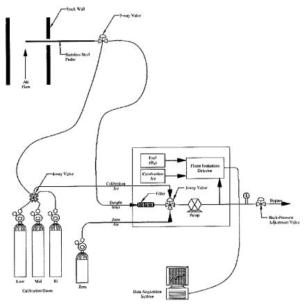
Figure 4-2. USEPA Method 25A Sampling Train
