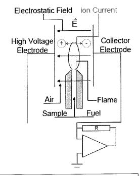
Figure 4-1. FID Flame Chamber
