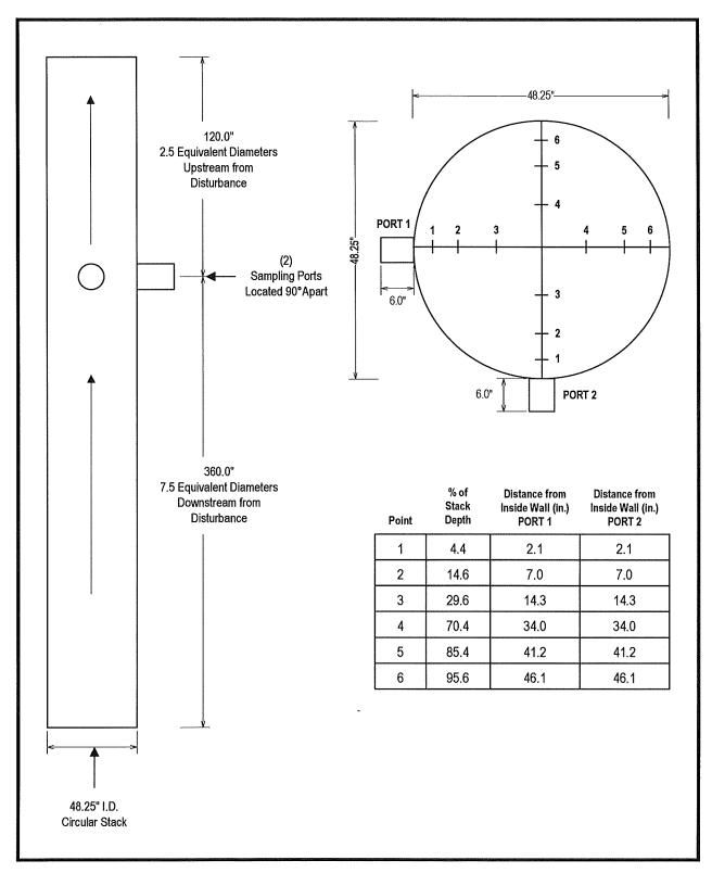
FIGURE 4-6 EU-ECOAT RTO EXHAUST STACK FLOW TRAVERSE SCHEMATIC
