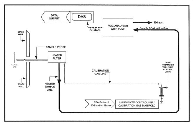
FIGURE 4-3 EPA METHOD 25A SAMPLING TRAIN
