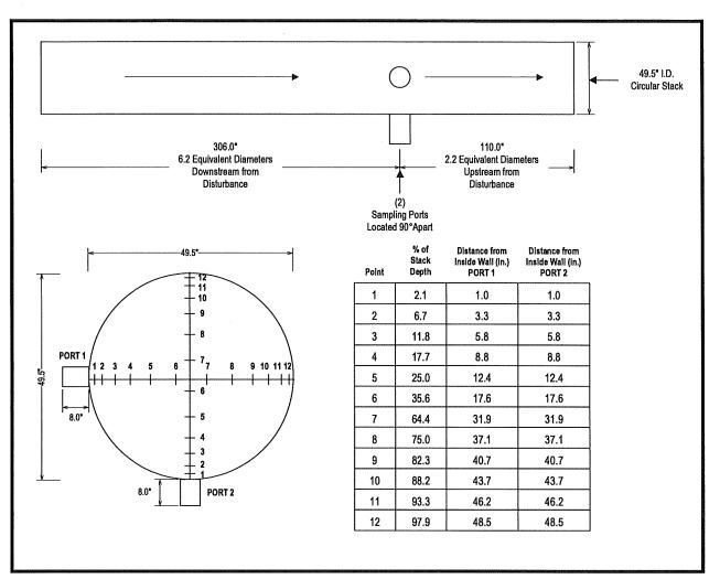
FIGURE 4-5 EU-ECOAT RTO OVEN INLET DUCT FLOW TRAVERSE SCHEMATIC
