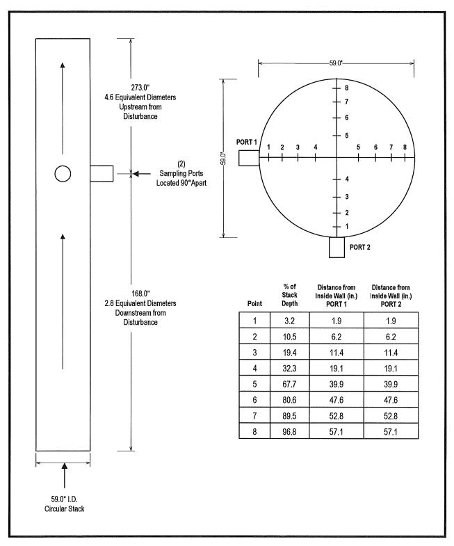
FIGURE 4-13 EU-TOPCOAT OVEN EXHAUST STACK FLOW TRAVERSE SCHEMATIC
