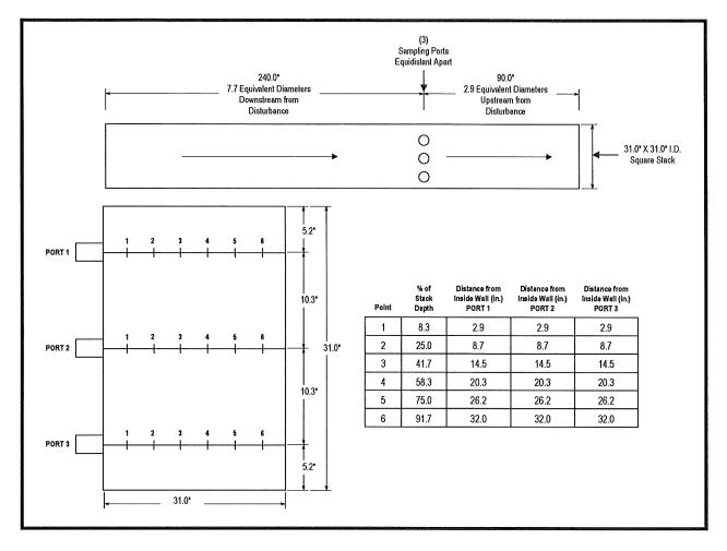
FIGURE 4-12 EU-TOPCOAT OVEN INLET DUCT No. 2 FLOW TRAVERSE SCHEMATIC
