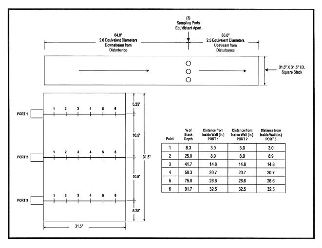
FIGURE 4-11 EU-TOPCOAT OVEN INLET DUCT No. 1 FLOW TRAVERSE SCHEMATIC
