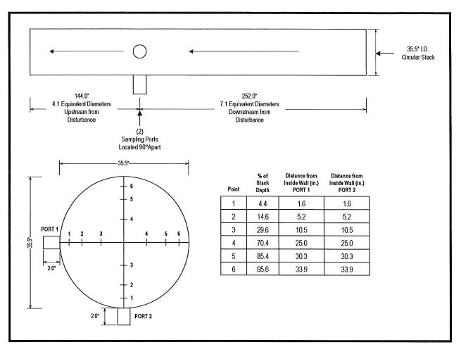
FIGURE 4-9 EU-TOPCOAT BOOTH #2 RTO INLET DUCT FLOW TRAVERSE SCHEMATIC
