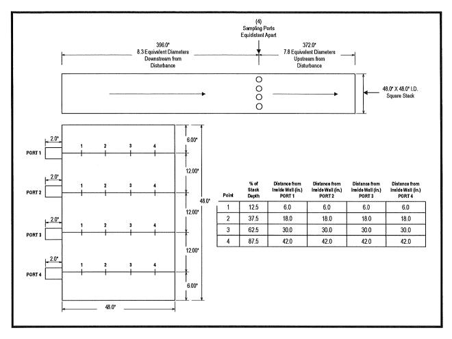
FIGURE 4-7 EU-TOPCOAT BOOTH #1 RTO INLET DUCT FLOW TRAVERSE SCHEMATIC
