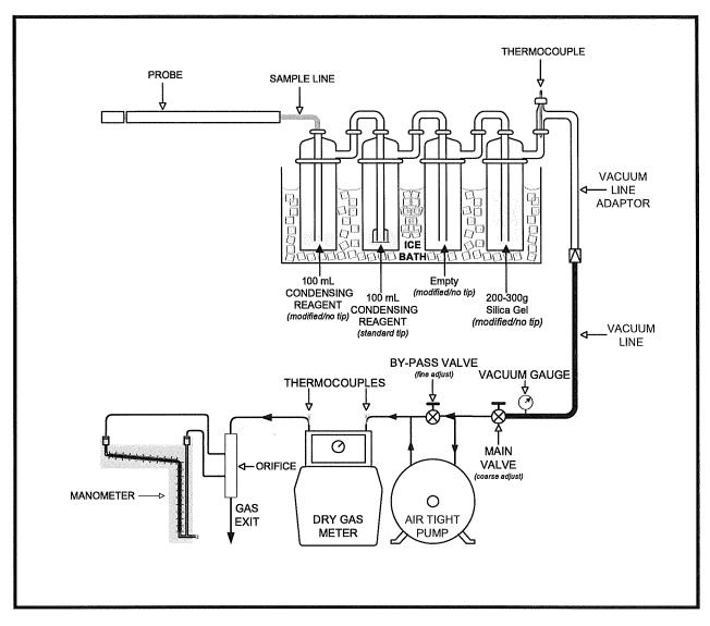
FIGURE 4-2 US EPA METHOD 4 (DETACHED) SAMPLING TRAIN
