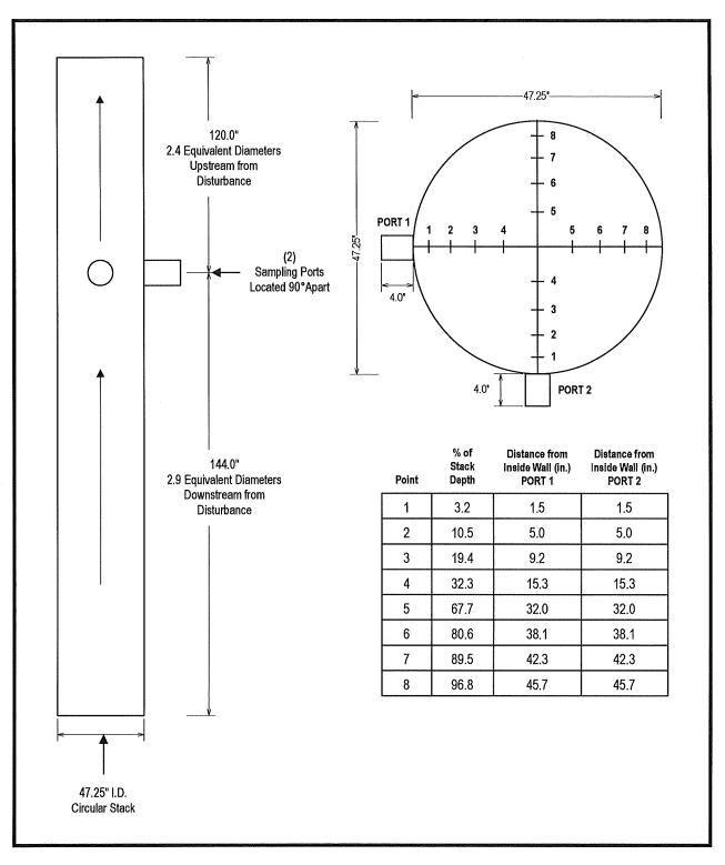
FIGURE 4-8 EU-TOPCOAT BOOTH #1 RTO EXHAUST STACK FLOW TRAVERSE SCHEMATIC
