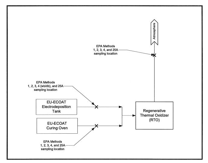
FIGURE 3-1 EU-ECOAT SAMPLING LOCATION SCHEMATIC
