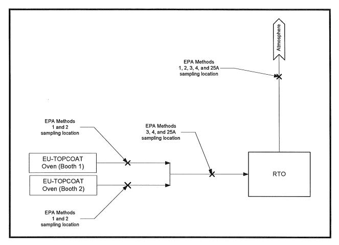
FIGURE 3-3 EU-TOPCOAT OVEN RTO SAMPLING LOCATION SCHEMATIC
