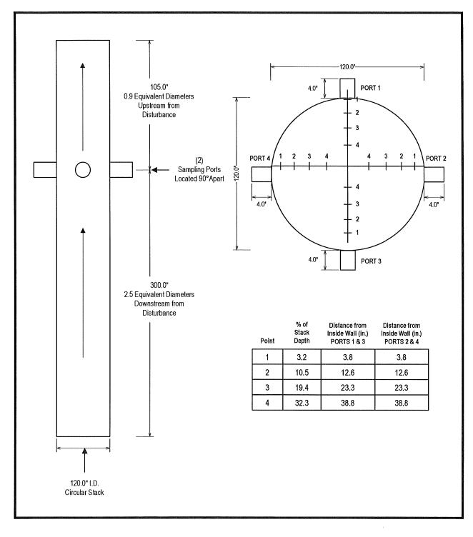
FIGURE 4-10 EU-TOPCOAT BOOTH #2 RTO EXHAUST STACK FLOW TRAVERSE SCHEMATIC
