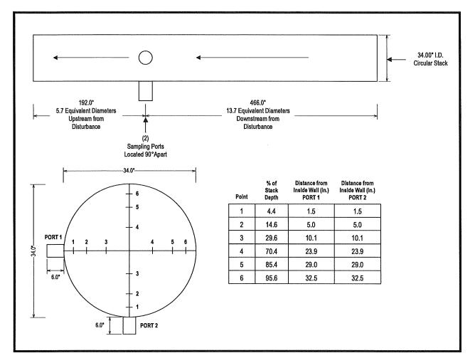
FIGURE 4-4 EU-ECOAT RTO TANK INLET DUCT FLOW TRAVERSE SCHEMATIC
