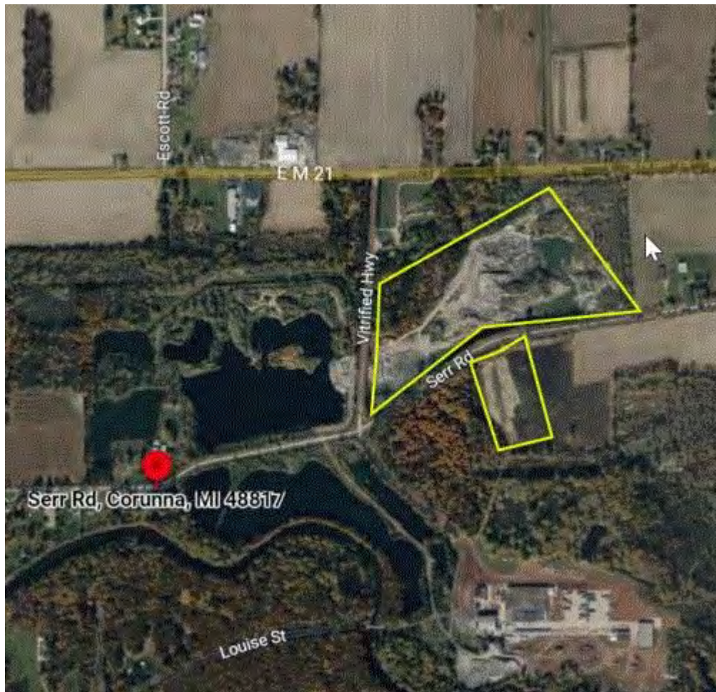
Image 1(Facility Aerial) : Yellow outlines indicate new (southernmost) and old (northernmost) shale mining pits.
