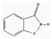
Table 1. Chemical properties of BITMolecular weight: 151.183 grams/moleMelting point: 156.6 °CBoiling point: 327.6 °CVapor pressure: 2.78 x 10<sup>-6</sup> mmHg at 25°CPhysical state at room temperature: solidReference: PubChem Compound Database
